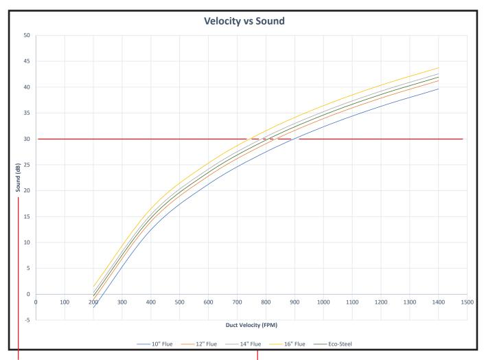
**Sound** vibration is measured in Decibels (dB). Utilizing 30 dB or lower as an acceptable noise pollution standard. We design our systems to stay below this level at peak exhaust fan speed.
