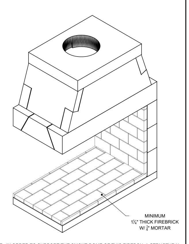
NOTE: IN ORDER TO SUPPORT THE SMOKE DOME OF THIS FIREBOX, A STRUCTURAL STEEL SUPPORT FRAME MUST BE DESIGNED AND APPROVED BY A STRUCTURAL ENGINEER. SMOKE DOME WEIGHT EXCLUDING MORTAR AND EXHAUST COMPONENT IS 648 LBS.
